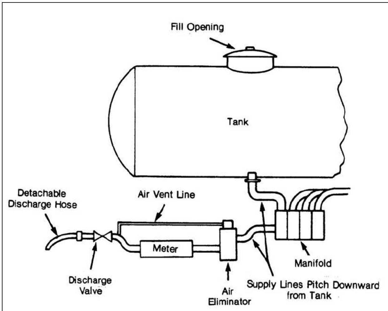
Figure 2-2. Diagram of a Gravity-Discharge System
