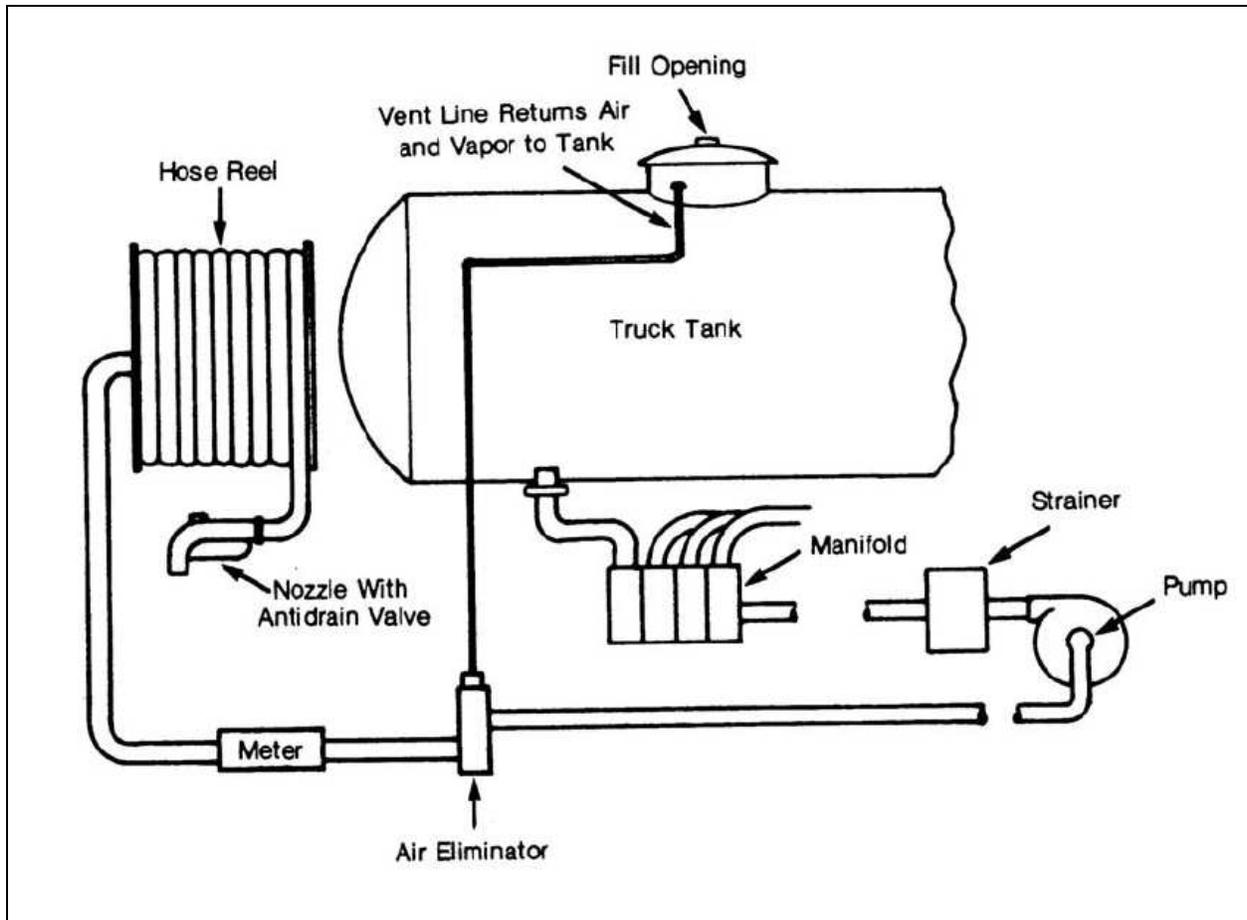
Figure 2-3. Power-Operated System
