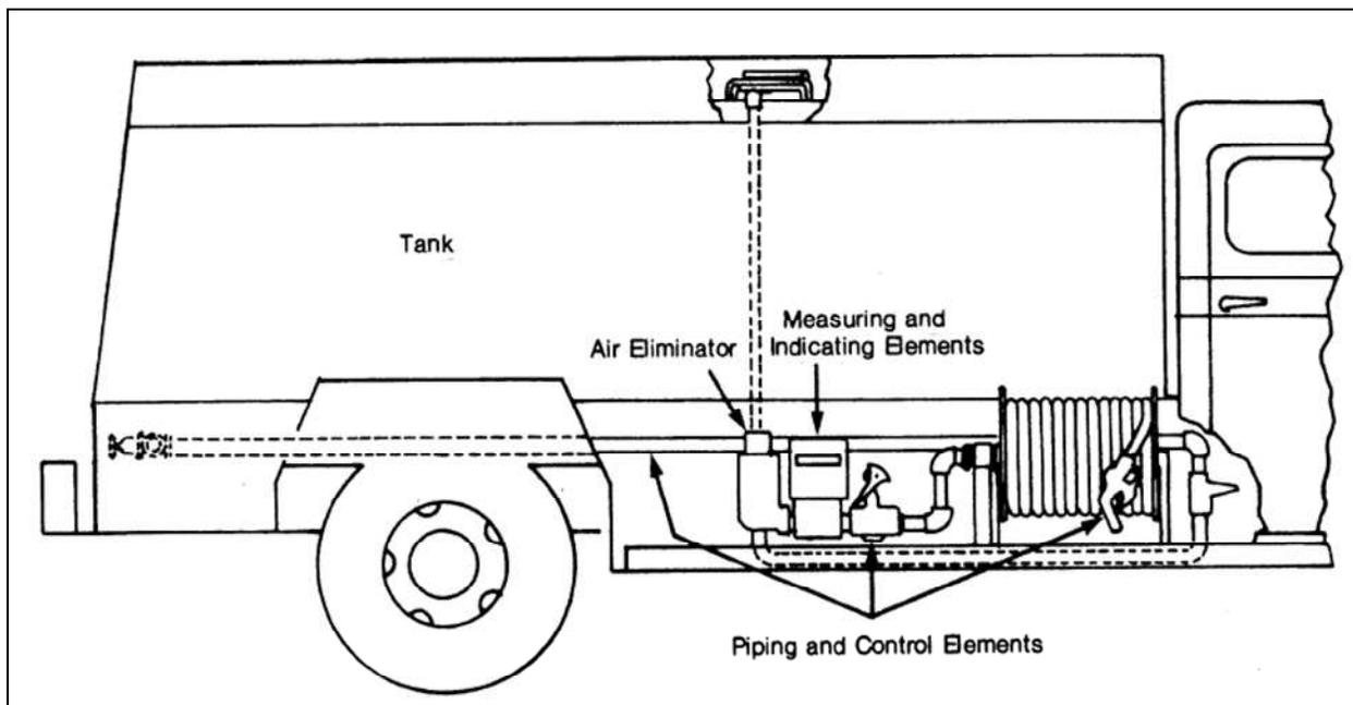
Figure 2-1. The Vehicle-Tank Metering System
