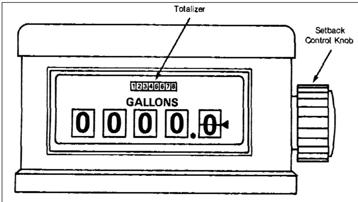
Figure 3-8. Mechanical Register
