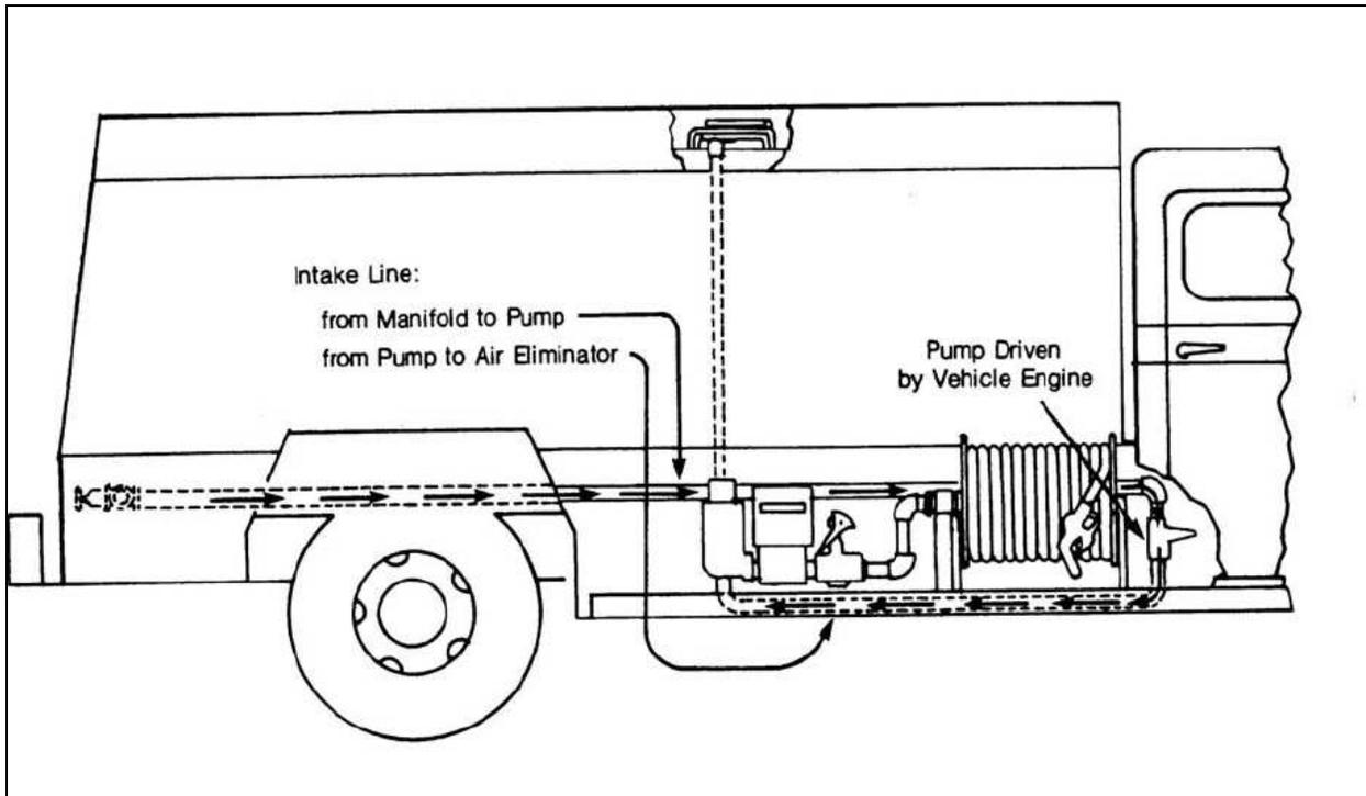
Figure 3-1. Power-Operated System
