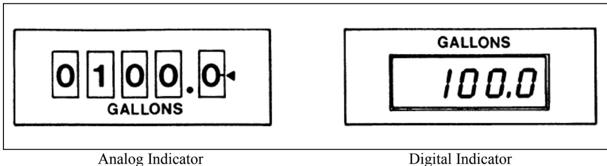
Figure 3-12. Analog vs. Digital Indications (I)
