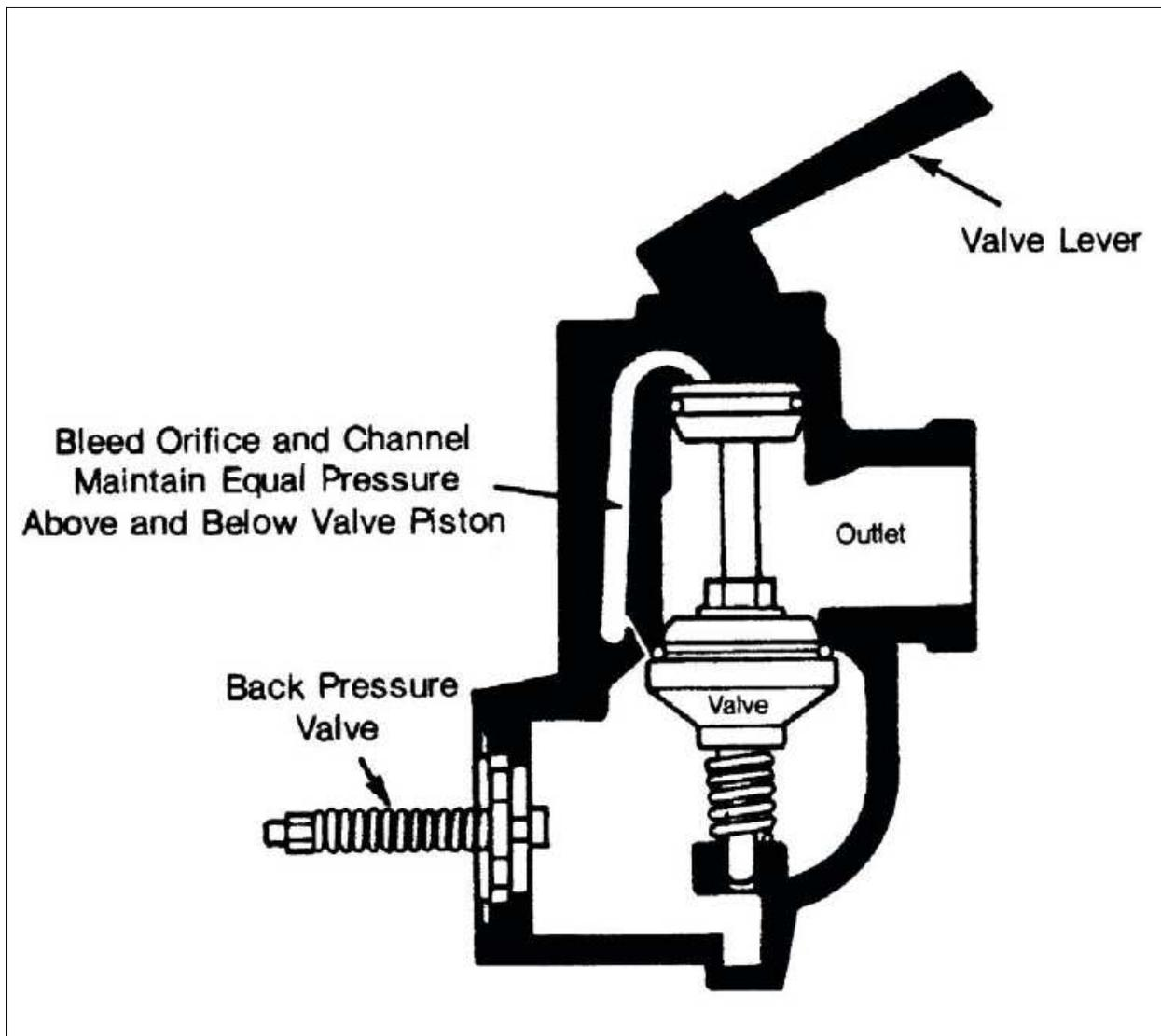
Figure 3-15. Cutaway Diagram of Control Valve
