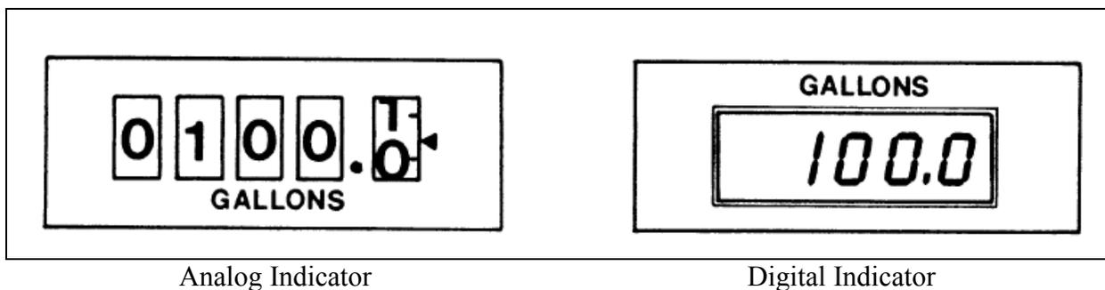
Figure 3-13. Analog vs. Digital Indications (II)
