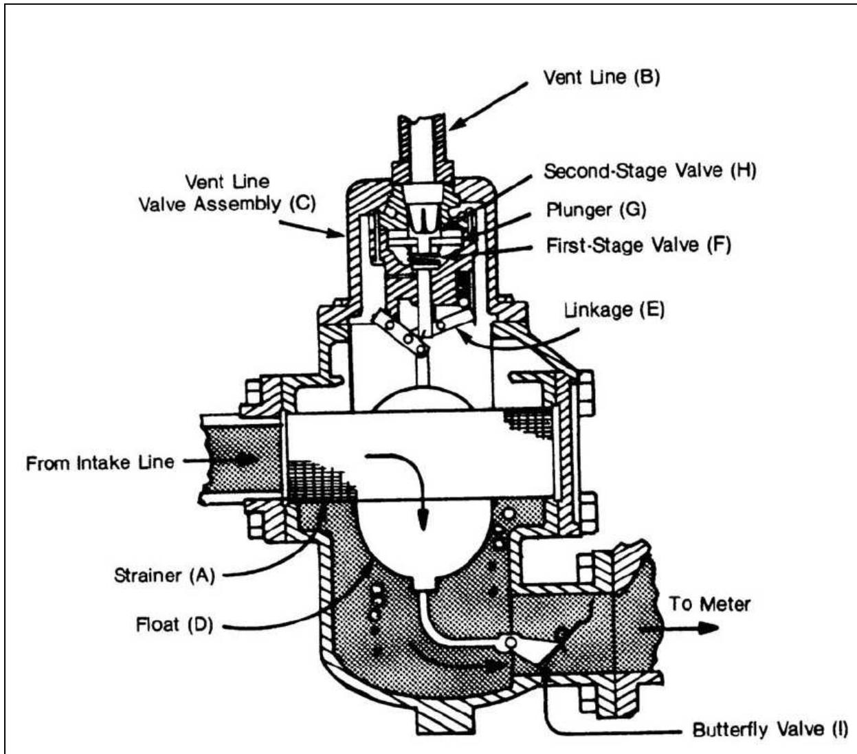
Figure 3-3. Cutaway of a Typical Air Eliminator
