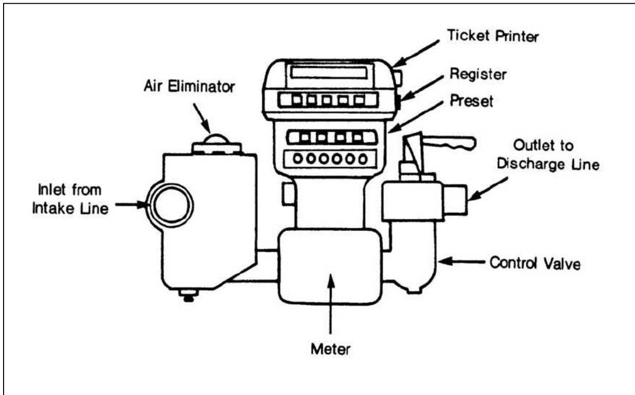
Figure 3-2. Air Eliminator and Meter Assembly
