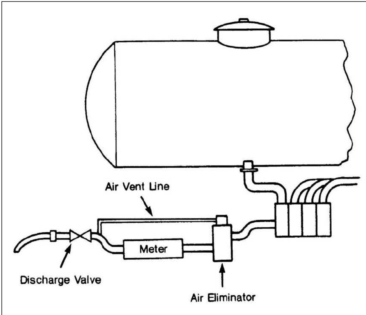
Figure 3-5. Installation of Vent Line, Gravity Discharge System
