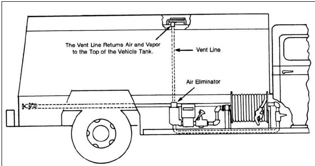
Figure 3-4. Installation of Vent Line, Power-Operated System
